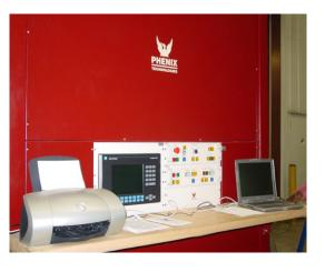
The area has also been equipped with a new Phenix Power Panel. With it, we will be able to closely simulate the conditions under which a motor operates in your facility. The variable voltage allows us to test from 0 volts to 4160 volts of AC power and 0 volts to 600 volts of DC power. It also will generate precise computerized readings for vibration levels, voltage and amperage.
